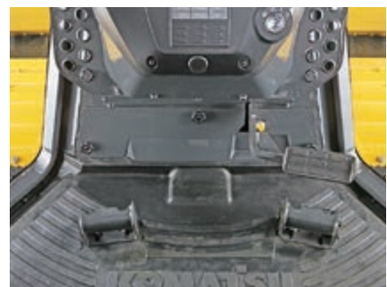
Combined decelerator/brake pedal
