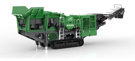
Optimized for Type 1 crushing applications, the J45 features a heavy-duty bofor design and transfer chutes with steeper angles to reduce material sticking.
