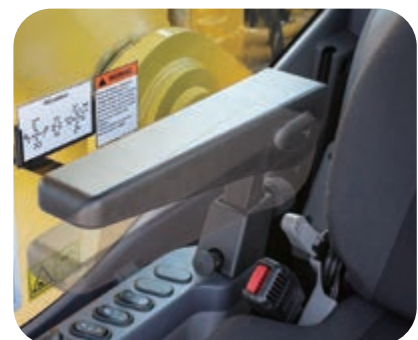
Armrest with simple height adjustment
