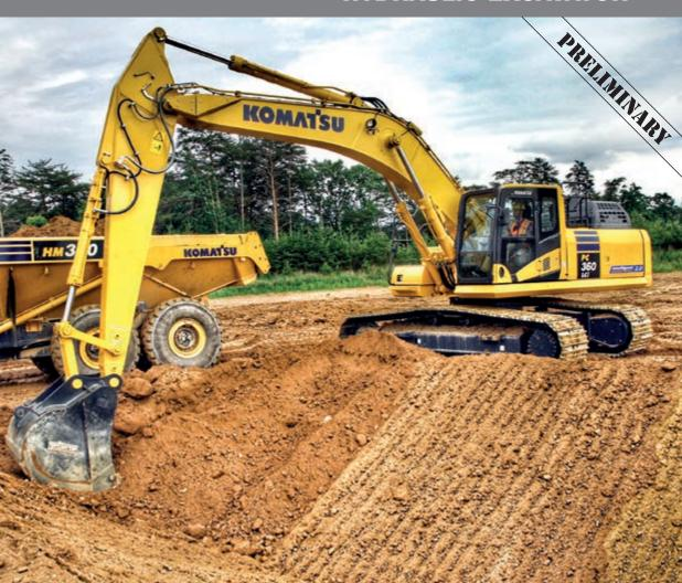
ENGINE POWER 202 kW / 271 HP @ 1.950 rpm **OPERATING WEIGHT** PC360LCi-11: 35.900 - 36.850 kg PC360NLCi-11: 35.770 - 36.530 kg BUCKET CAPACITY max. 2,66 m<sup>3</sup>
