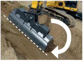
**New Auto Tilt Control** Automatically tilts bucket to design and returns it to horizontal to unload. Makes delivering final grade quicker and easier.
