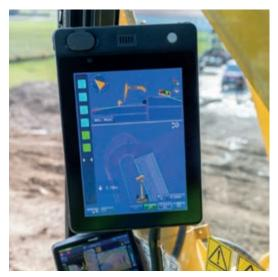
**New 10,4" iMC monitor** Slimmer, lighter and more compact, with increased memory capacity and processing speed. Positioning, mounting and dismounting are easier than ever.
