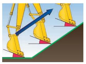
New bucket angle hold feature Operator selects desired bucket angle and the system maintains bucket angle through grading pass. Vastly increases ease of operation on final grading and trimming work.
