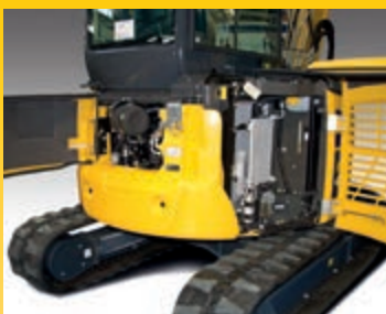
Rear bonnets for quick engine checks, simple inspections, cleaning of the radiators and easy access to the battery
