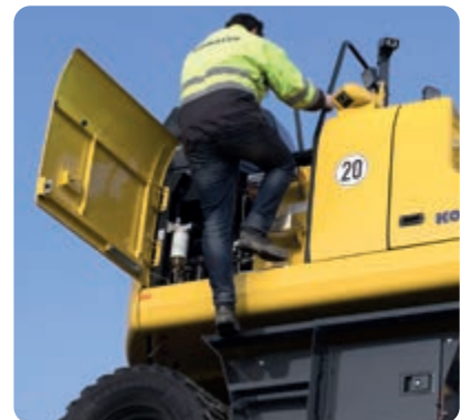
Handrails and anti-slip plates
