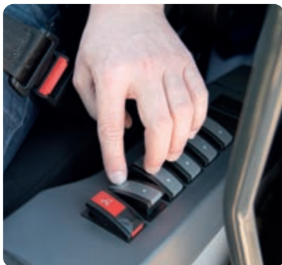
Ergonomically designed switches that light up for safe and easy night operation
