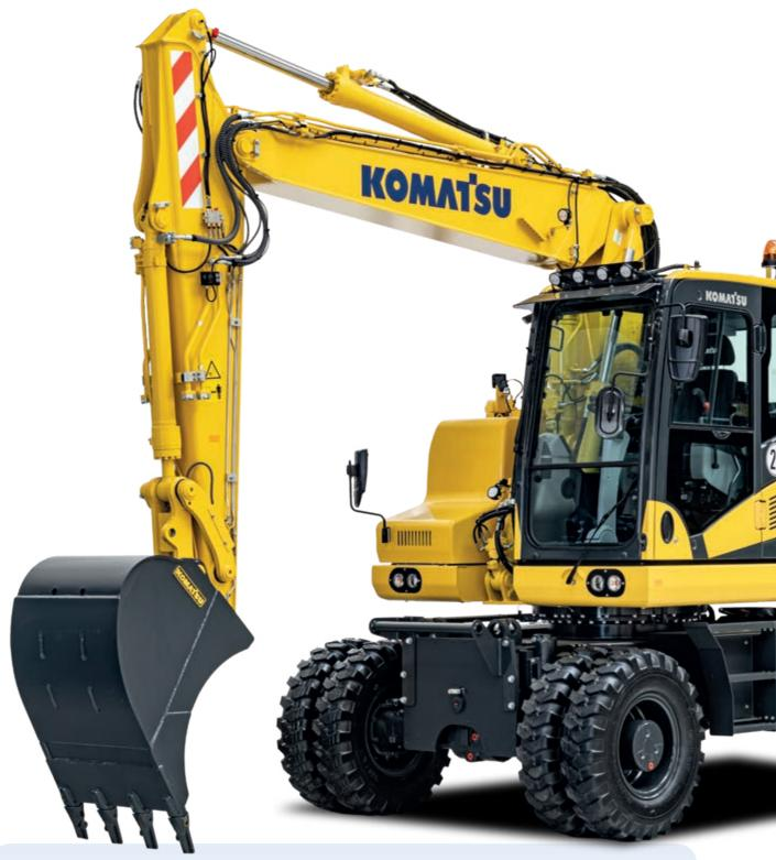
Engine power 110 kW / 148 HP @ 2000 rpm
