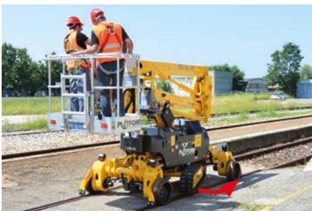
The 90 deg tracks swiveling enable an easy and quick in & out from railway track.
