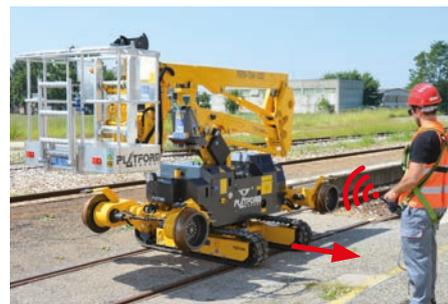
Driving of the machine can be operated by a remote control unit fitted on board of the basket or by the operator at ground with no load in the basket.
