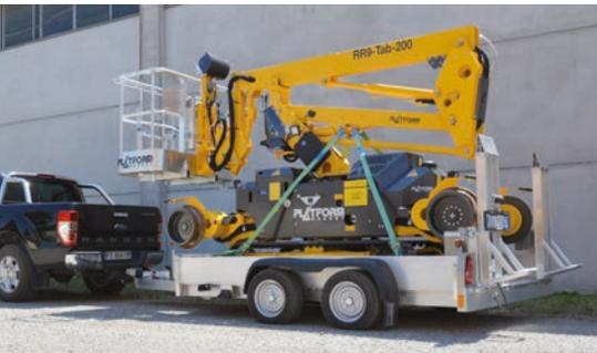
**The structure** of the RR9/200 is composed of an base car designed on track for road and off-road use that offers excellent grip on the ground in any ground condition together with a low specific load particularly designed to allow its movement even in the presence of delicate floors of railway stations.
