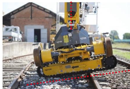
**The power** is delivered through a diesel endothermic engine of 10.5 KW power, on request it will also be possible to equip it for fully electric operation with lithium-ion batteries in order to make the equipment suitable for use in tunnels, subways and inside buildings such as hangars, stations, etc.
