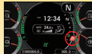
AdBlue® level gauge and refill guidance
