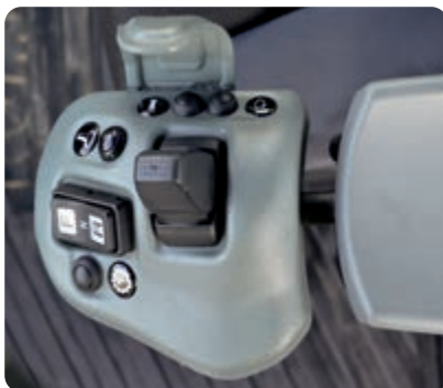
Komatsu Short Lever Steering (K-SLS) (option)
