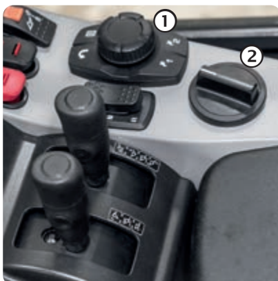
Komatsu Short Lever Steering (K-SLS) (option)
