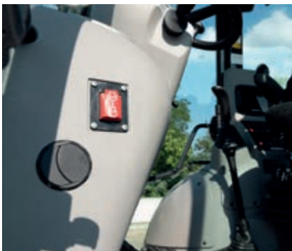
Secondary engine shut down switch
