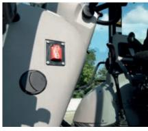
Secondary engine shut down switch
